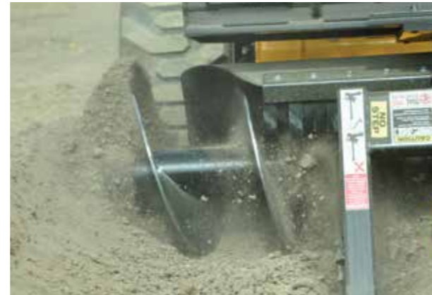
Powered by a compact DIGGA planetary gearbox and EATON hydraulic motor, your guarantee of quality and superior performance.
